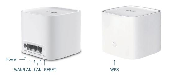
• Wireless Standards: IEEE 802.11a/n/ac/ax 5GHz, IEEE 802.11b/g/n/ax 2.4GHz • Signal Rate: 5 GHz: Up to 1201 Mbps, 2.4 GHz: Up to 574 Mbps • Transmit Power: FCC: <30 dBm, CE: <20 dBm (2.4 GHz), <23 dBm (5 GHz) • Wireless Function: MU-MIMO, Beamforming, Band Steering, Airtime Fairness · Wireless Security: WPA/WPA2/WPA3 Personal, WPA/WPA2 Enterprise
